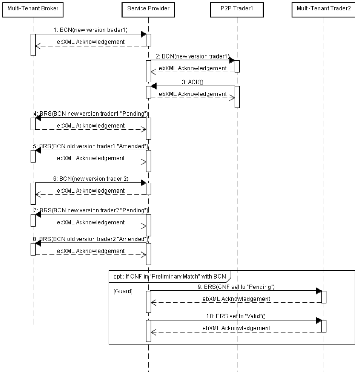
Figure 17 Document flows for amendment of the Broker Confirmation in the Trilateral Matching dialogue
